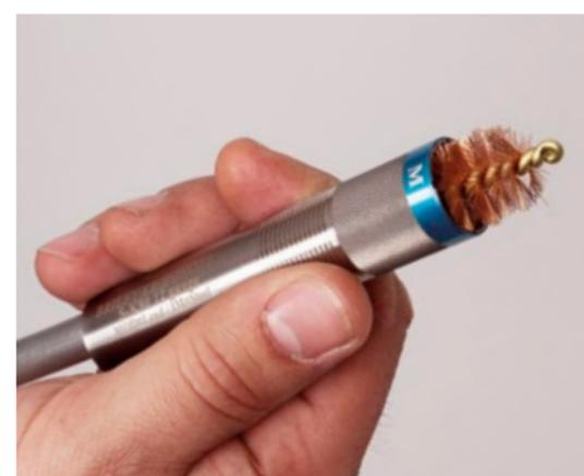
After cleaning it is very important to spray the choke tubes completely with a thin gun oil to prevent corrosion.
